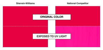
Here, Exterior Accents and a national competitor were each applied to identical panels. Part of each panel was covered, and the panels were exposed to accelerated high intensity UV light that represents sunlight. When the covered portion was revealed, the result was clear: Exterior Accents is more resistant to the fading effects of UV rays.
