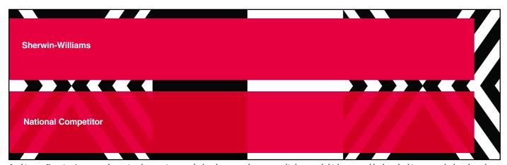
In this test, Exterior Accents and a national competitor matched to the same color were applied at equal thickness over black and white test cards that show the relative hiding power of each coating. The competitors' product is transparent, with the black and white stripes clearly showing through the dried film. The result is undeniable: Exterior Accents hides better.
